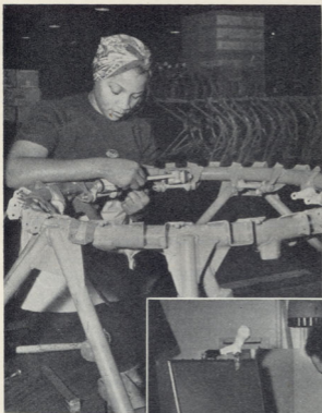
Assembling a bomber motor mount.
